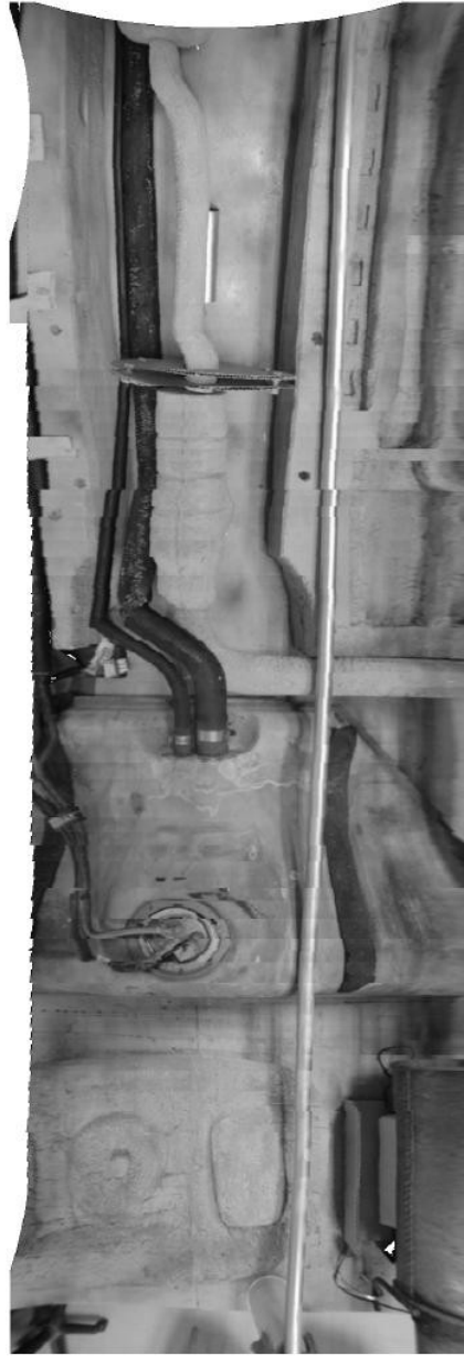
Figure 16. A straight line motion test. The mosaic is made from one camera moving down the length of the mockup in a straight line at constant speed. The straight piece of PVC pipe was laid on the mockup to test the ability of the system to reconstruct straight objects.
