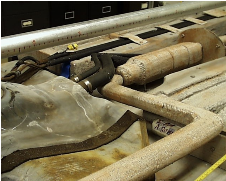
Figure 13. A close-up picture showing the 3D structure of the mockup parts. Notice the suspicious item under the tailpipe near the lower right corner.
