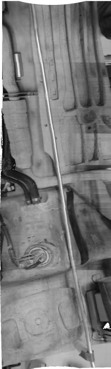
Figure 17. Angled straight line motion test. The mosaic is made from one camera moving down the length of the mockup at a fixed angle at constant speed. The straight piece of PVC pipe was laid on the mockup to test the ability of the system to reconstruct straight objects.
