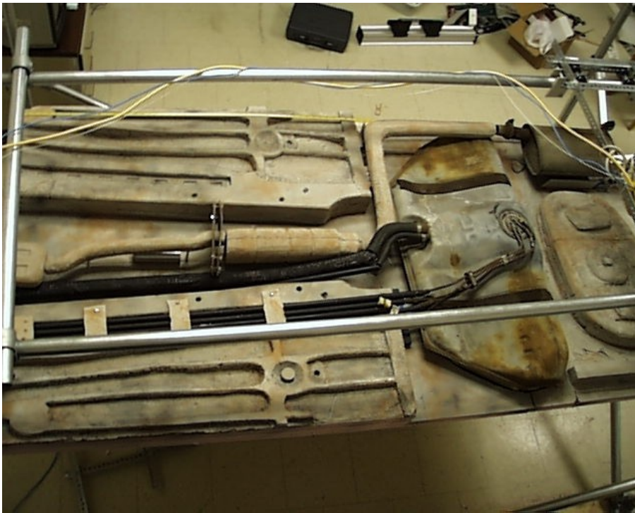
Figure 12. A picture of the undercarriage mockup built from car parts as well as Styrofoam and cardboard pieces
