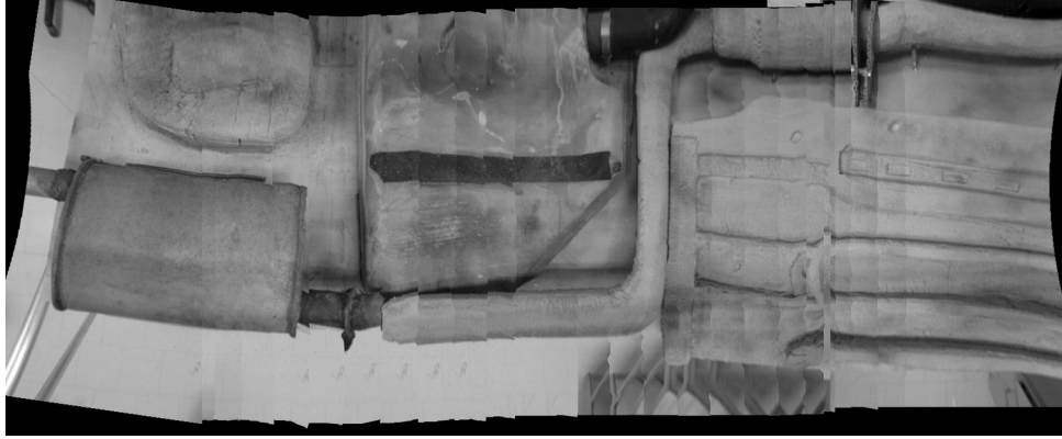
Figure 10. The 3D mosaicing result of image sequence with 3-inch camera distances (50-pixel image motion on average). The mosaic is not perfect but is good enough for understanding the under-vehicle.
