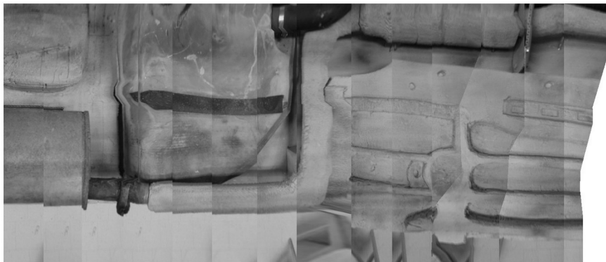
Figure 12. The 3D mosaicing result of image sequence with 6-inch camera distances (100-pixel image motion on average). The “camera locations” of the moving camera was estimated by a simple calibration procedure with metric measurements of the camera movements, and the local matches were established manually. The result shows that if we can develop an effective local matching algorithm for view interpolation, we can still make good image mosaic with rather sparse camera array (e.g. 6 inch apart).
