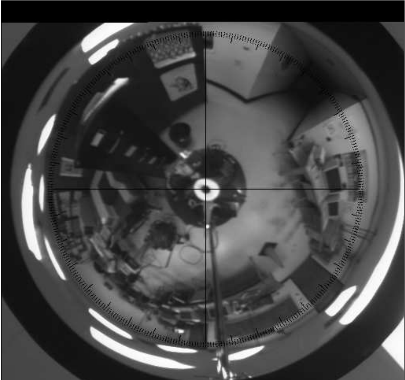
Figure 2: (b) A sample image taken in our experiment. The white ring indicates the rotation center of the robot and the marked ticks are the horizon circle, together with the coordinate axes
