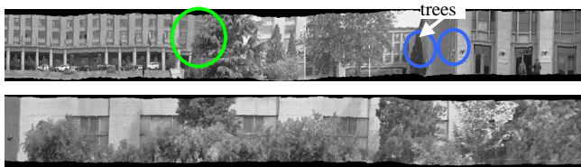
Fig. 6. Multi-viewpoint mosaic with adaptive time scales (The right edge of the upper part connects with the left edge of the bottom part). The width of each vertical slice from the corresponding original frame is determined by the dominant image velocity v of pixels along the y -axis in the corresponding PVI. Circles show the corresponding OCCLUDED and SIDE regions in Fig. 5.
