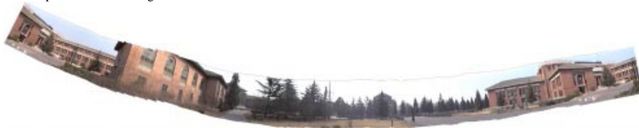
Fig 5. Flattened conic mosaic (13% display scale). The original color image is 3806 x 773x24 bits. Notice the curved and uneven boundary created by the up-tilted angle and unstabilized motion of the hand-held camera, and error accumulating.
