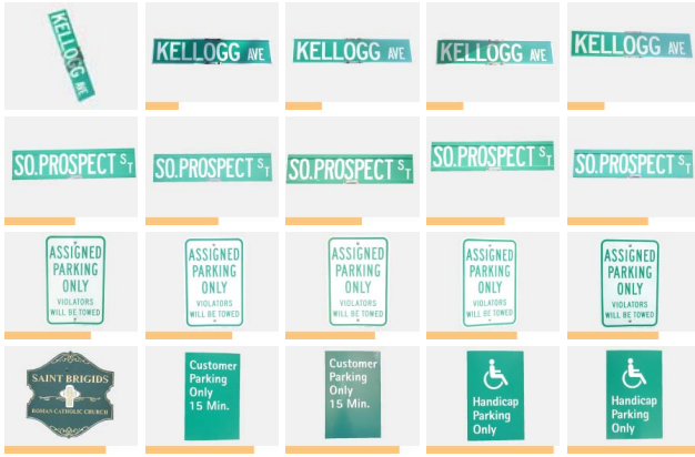
Figure 6. An example of ranking results by the matcher. The image in the upper left corner is the query, the remaining 19 images are the matches in rank order: rank 1-4 on the first row, 5-9 on the second, 10-14 on the third, and rank 15, 19, 23, 27, and 31 on the fourth row. The length of the bar on the bottom of each sign represents the matching cost.
