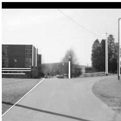
Figure 22: Projection of model for outdoor frame 3 using final estimate of Algorithm “Med_R_and_T_mod” with high prior covariance matrix.
