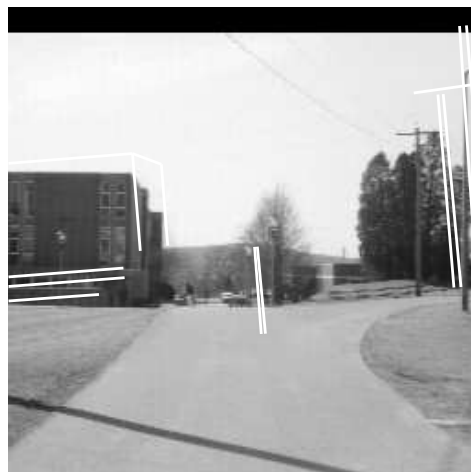
Figure 21: Projection of model for outdoor frame 3 using final estimate of Algorithm “R_and_T_mod” with high prior covariance matrix.
