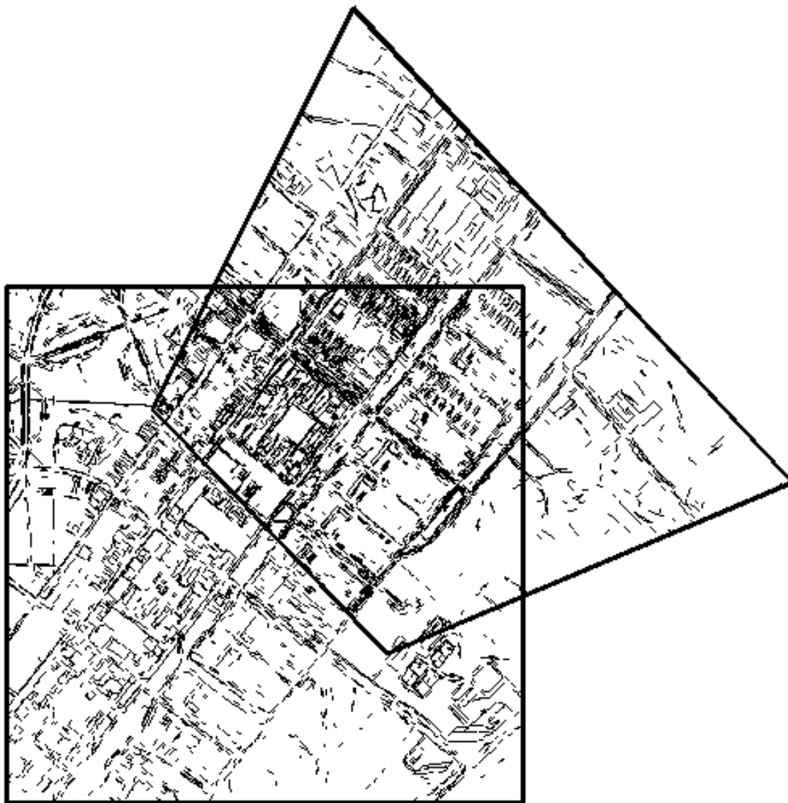
Figure 4.11: A final registered mosaic for the two images in Figure 4.10. Line segments from the oblique view have been projectively unwarped into the coordinate system of the nadir view.
