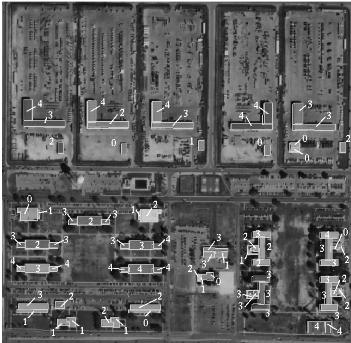
Figure 15: The ground truth model projected into image 713. The number of times each roof polygon was detected over the four different views is overlaid to depict an overall 2D detection rate of 89% for batch-mode processing at 0.7 sensitivity setting.
