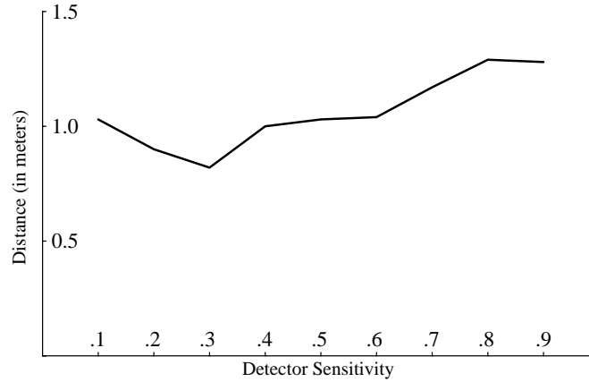
Figure 18: Building detector sensitivity vs. 3D polygon accuracy, computed as the median of center-line distances between reconstructed 3D polygons and ground truth polygons
