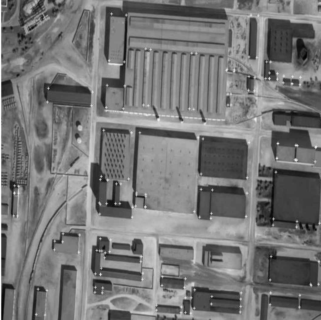
Figure 9: Extracted image points in image J3. The 186 points are a result of generating 2D building polygons via the ASCENDER system.
