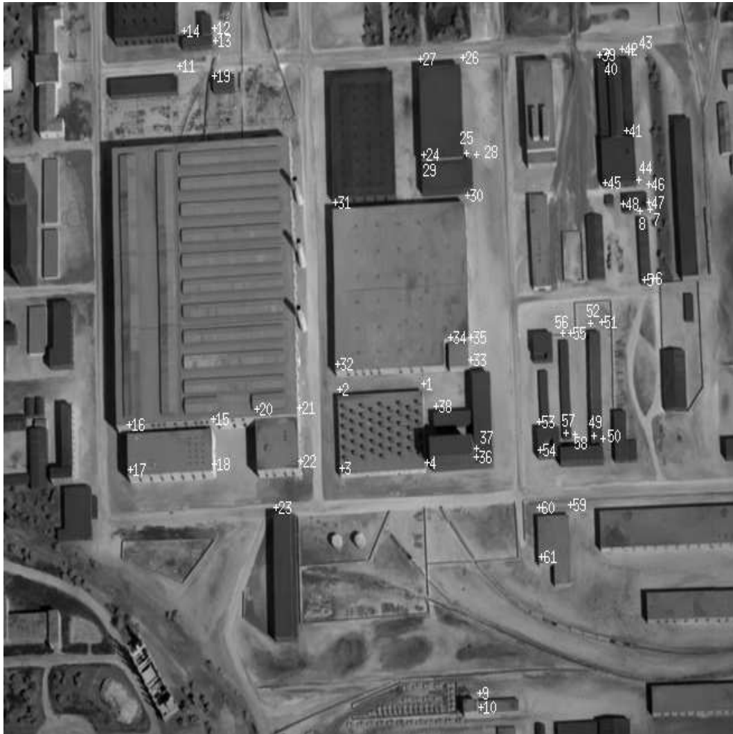
Figure 12: Experiments with RADIUS detect 61 matched image points in image J7.
