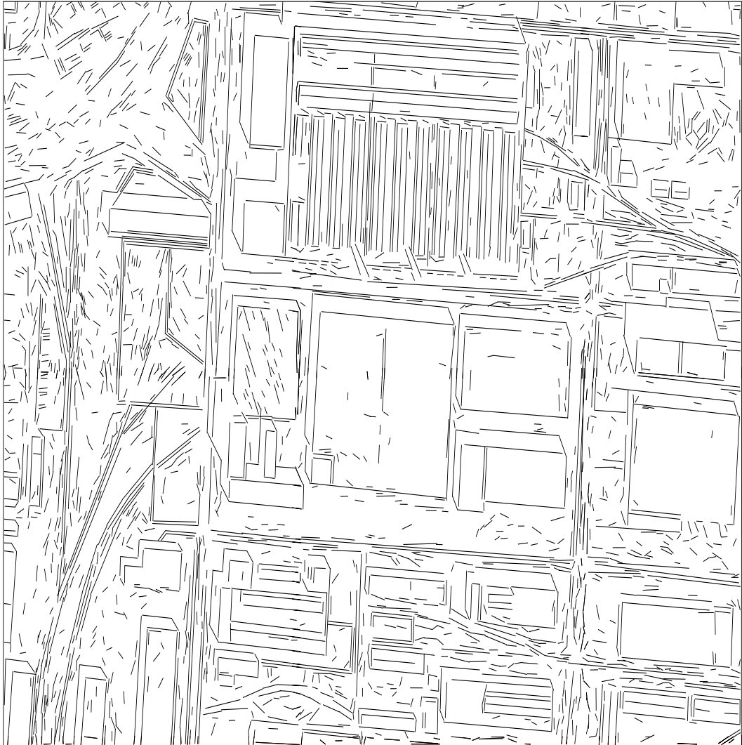
Figure 18: RADIUS model board image J3. The Boldt straight line extraction algorithm produced 2734 lines.
