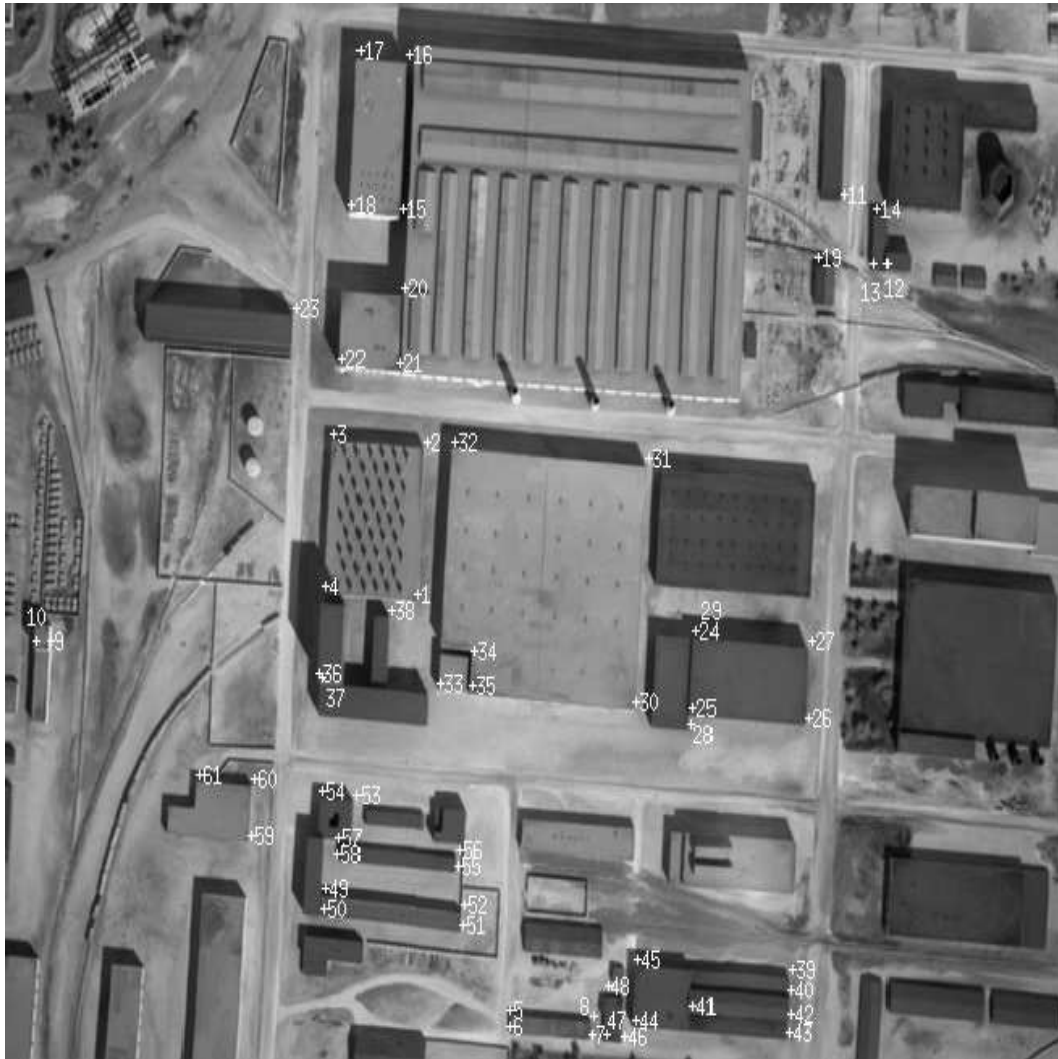
Figure 11: Experiments with RADIUS detect 61 matched image points in image J3.
