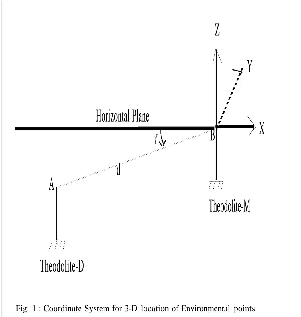
Fig. 1 : Coordinate System for 3-D location of Environmental points
