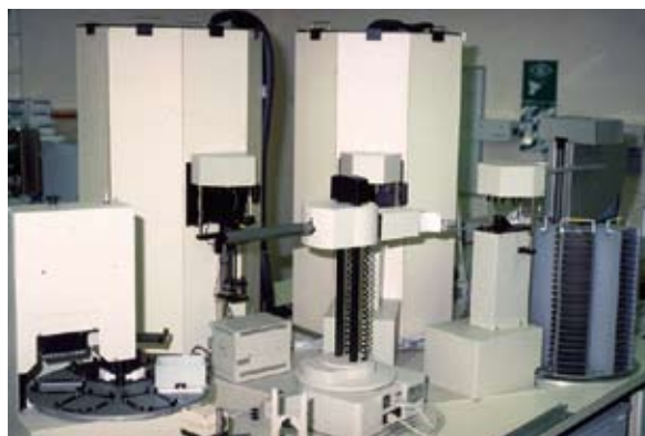
Figure 4. High throughput screening robot. Many analytical techniques that are developed on a small scale have now been modified to deal automatically with large numbers of compounds in screens for potential drugs that will contribute to pharmaceutical exports. This means that, for example, a million compounds may be screened for biological activity in just a few months.
