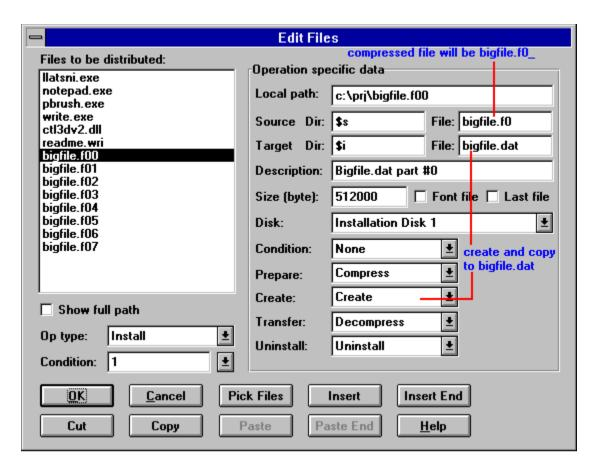
Note that because bigfile.f00 is the first part of bigfile.dat, we use the create mode to create bigfile.dat on the user's system. For all other parts, we will use append mode to append the bigfile.dat created by bigfile.f00.
