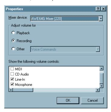
Now when you click "OK" you will see a Recording Control allowing you to adjust the volume for Line-In and Microphone recording. Select either Line-In or Microphone inputs here depending on the audio source that you intend to use. It is best not to choose both inputs simultaneously, but to choose one or the other depending on the audio source.
