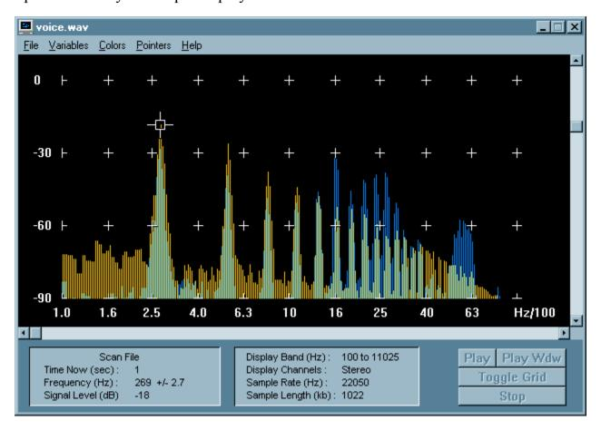
Spectrum Analyzer Scope Display – 1/3 Octave
