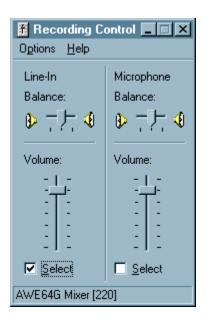
Occasionally this Recording Control will also have an active menu item "Options – Advanced Controls." If this menu item is available it should also be selected. This selection will make available an "Advanced" button on the Recording Control for turning Automatic Gain Control (AGC) on or off. AGC is often useful to keep the recording level automatically within the correct range.
