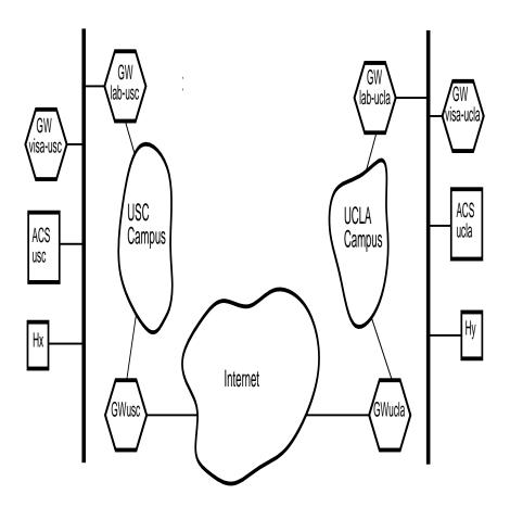
Figure 4: Internet configuration. Physical connections between USC and UCLA visa networks.
