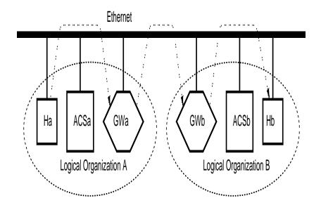
Figure 3: Laboratory configuration. Logically separate networks on a single physical network.
