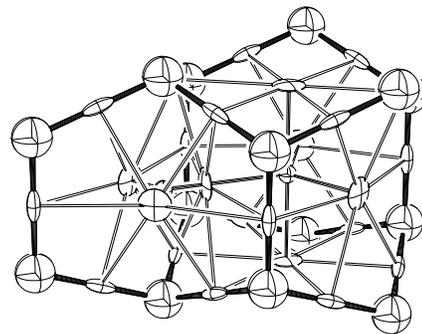
Figure 3.3. Critical net illustration of hexagonal diamond.
