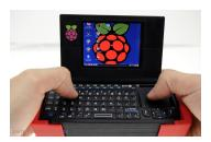
berry Pi single-board computer, Parts-people.com has an article describing how to build a mobile Pi-to-Go. It features an LCD screen, battery pack, internal powered USB hub, SSD storage, built-in WiFi & Bluetooth, and a mini keyboard & touchpad. You can even download an STL file to print off your own case for it, if you happen to have a 3D printer kicking around. Aside from the case, all other parts are available for purchase from various sites, for less than \$400.
