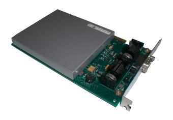
The Coprocessor includes sensors to protect against attacks involving probe penetration, power sequencing, radiation, and temperature manipulation . . .
