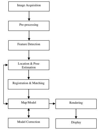
Figure 6. Flow chart describing the steps from the image acquistion to the tree model generation.
