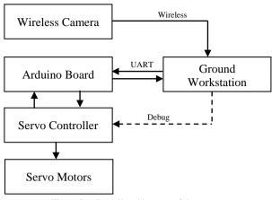
Figure 3. Overall architecture of the system.
