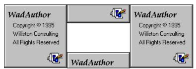
By default, the below texture is mapped from top to bottom, while the above texture is mapped from bottom to top. If this seems fairly innocent, consider the illustration to the left, a simple example of a window. A window is usually a small sector whose floor and ceiling are higher and lower than the surrounding sectors. In this event, the textures will be improperly aligned with the surrounding non-windowed walls.
