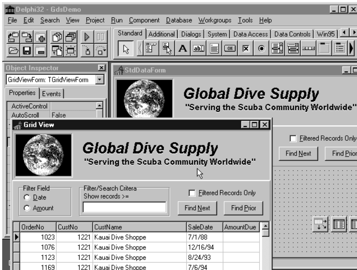
Figure 12 -- Delphi's Visual Form Inheritance allows you to easily create reusable, shared forms
