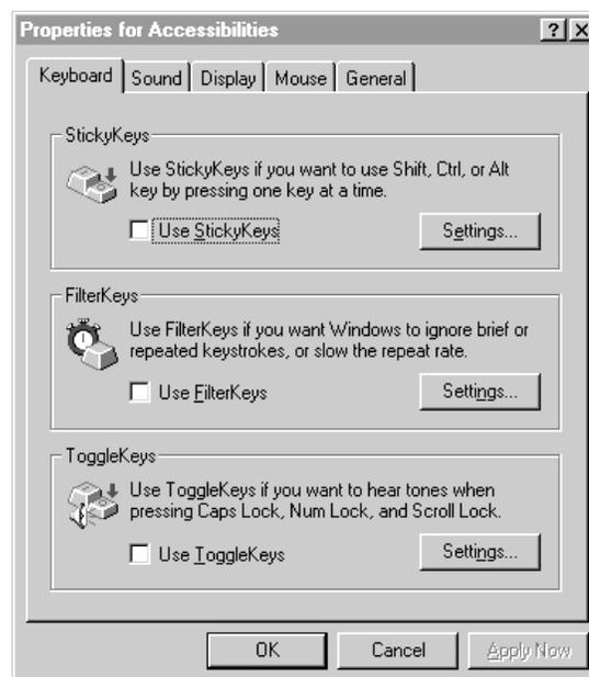
**Figure 1. The Accessibility Features property sheet in Control Panel**
