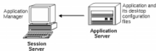
Figure 5-5 Standard application server configuration
