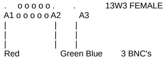
That's the coax part. The outer shielding of the coax's are grounded on both pin 10 and the case.
