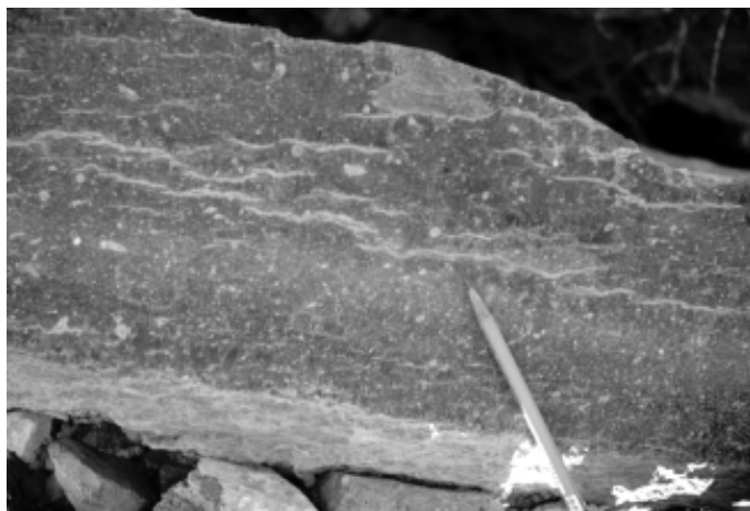
Figure 10. En échelon tension fractures in devitrified Huckleberry Ridge Tuff in Zone 2, near the bottom of the concrete boat-ramp just east of the Teton Dam. These fractures were filled with vapor phase crystals during subsequent cooling of the tuff. Most of these fractures dip gently to the northeast (left) in this area, indicating that the lower part of the unit moved to the southwest.
