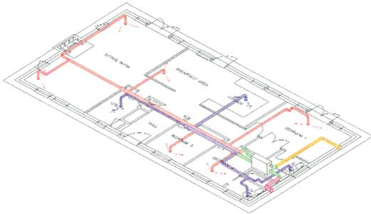
Ducting connects the stale air exhaust grille to the Heat Recovery unit and extracts via ducting to all the wet areas of the property. The stale air passes through the cross-flow heat exchanger and typically 65-70% of the heat normally lost via trickle vents is recovered.
