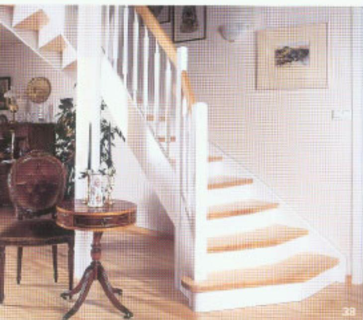
Quarter-turned, angled and widened base. Treads and handrail in beech. White strings, risers, spindles and newel post. Spindle no. 9 and post type D.
