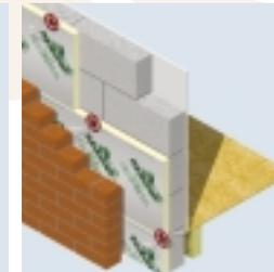
Boards are installed as work proceeds
