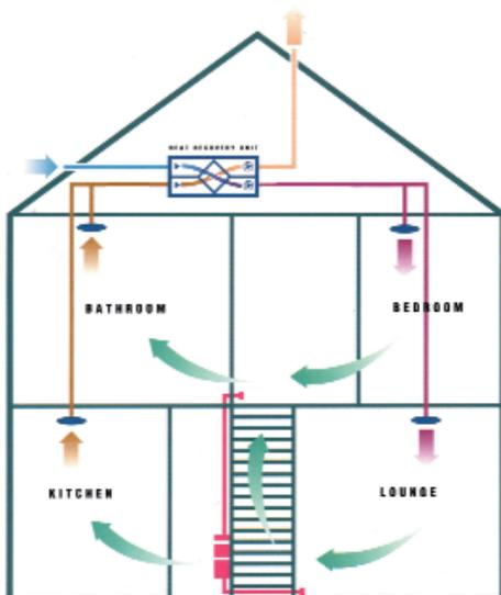
The Villavent Heat Recovery system is designed to completely change all the air in the property at least once every two hours, continually replacing the stale damp air with fresh, warmed clean filtered air.
