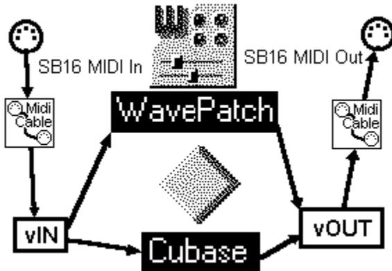
The TB-RIO card is hooked up as Waveblaster at the SB16-MIDI Ports (In and Out). Both programs, Cubase and WavePatch should have access to the Rio.
