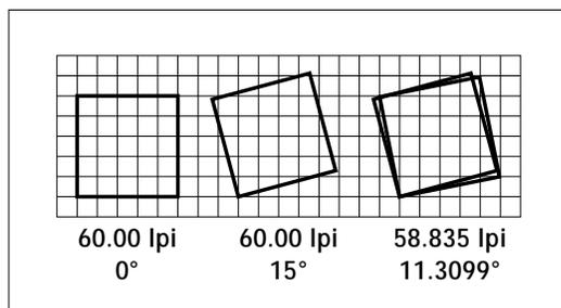
*Screen adjustments necessary for digital halftones on a 300-dpi device. To align with the nearest device pixel, the halftone cell angle must be adjusted. Adjusting the angle alters the number of pixels per cell, changing the actual cells per inch (lpi).*
