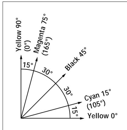
*Traditional screen angles. Slight moirés are produced by the 15-degree angle between yellow and magenta and yellow and cyan. Yellow is chosen for this rotation because it is the lightest color and therefore produces the least noticeable pattern.*
