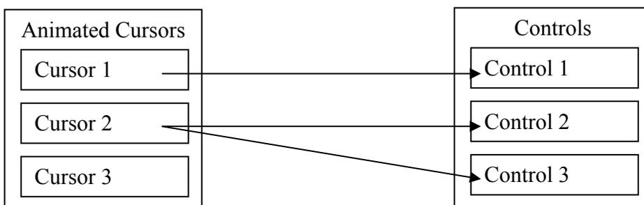
In this example, Cursor 3 is unused, but still available. Please note that Controls collection is not pre-initialised. You simply add control names to it. Also the names are not checked – you can add any name you like, but the cursor will only be applied if it is the name of a control on the form. Control arrays are
