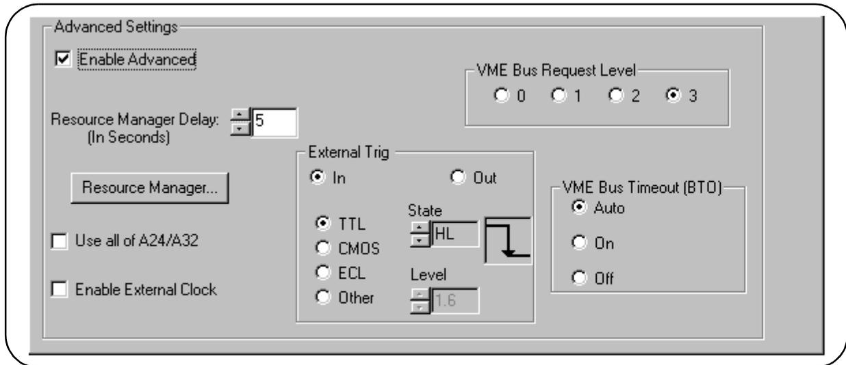
**Figure 3-1. Configuring the HP E8491B External Trigger Ports.**
