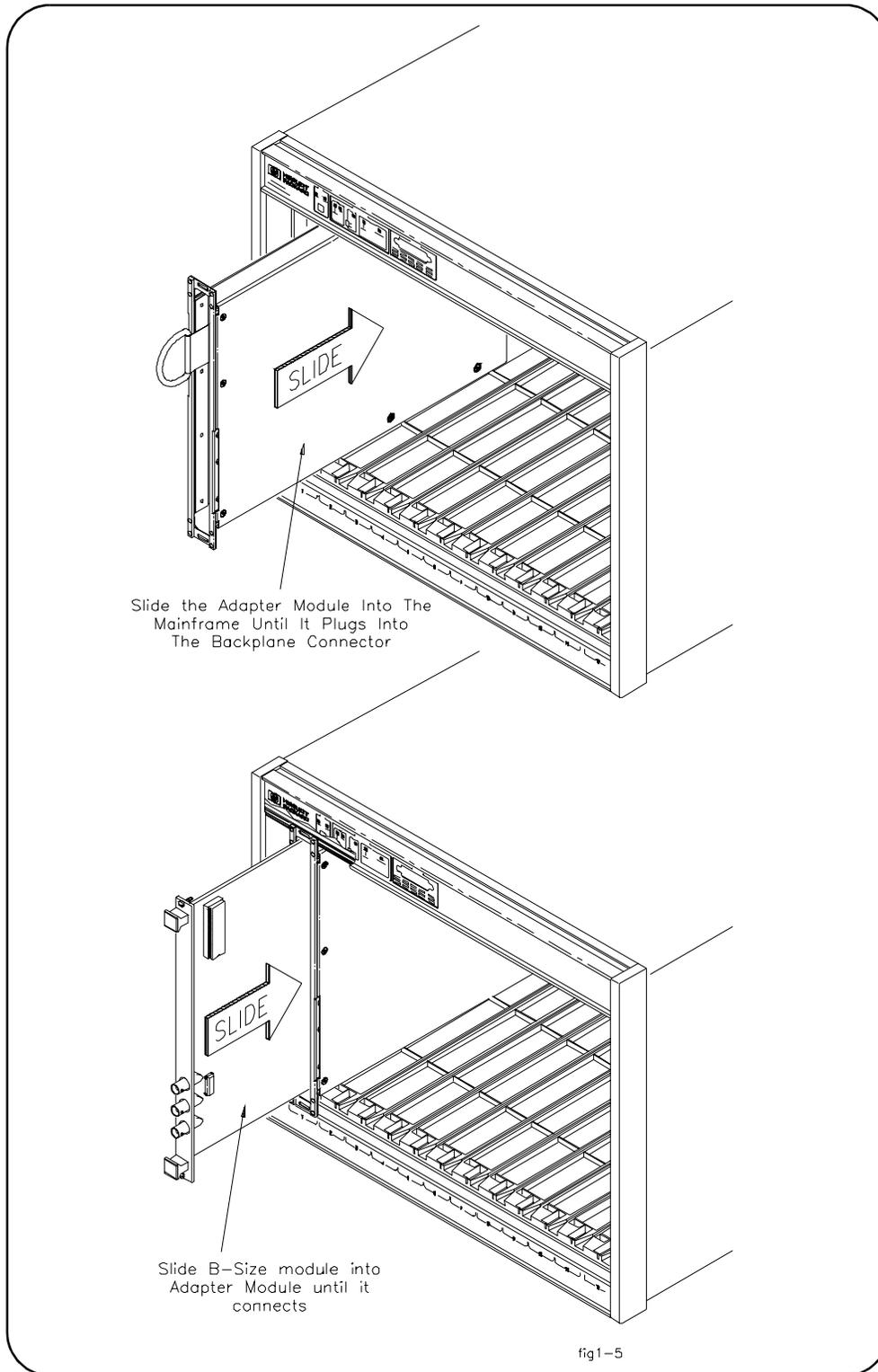
**Figure 2-9. Installing A- and B-size VXI Instruments.**
