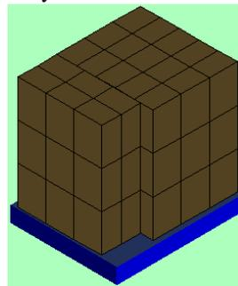
The user will note that some boxes may allow four configurations (numbered 1 to 4), which are the #1 and #2 (previously explained) and the #3 and #4 which are the result of optimizing the #1 and #2, respectively. Whether #3 or #4 deliver more boxes, depends on the box and pallet dimensions.
