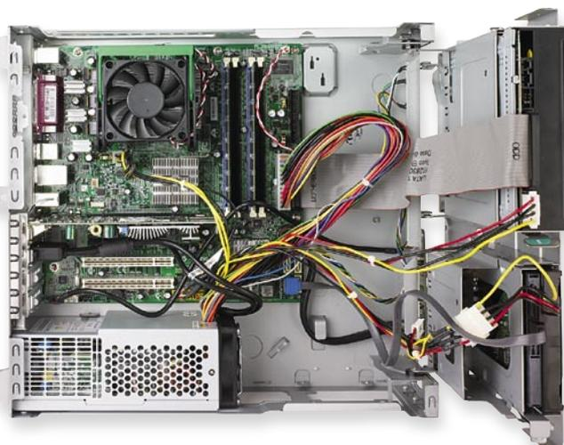
Inside the ML7, there's plenty of room for expansion and it's relatively easy to work on thanks to the tool-less drive racks.
