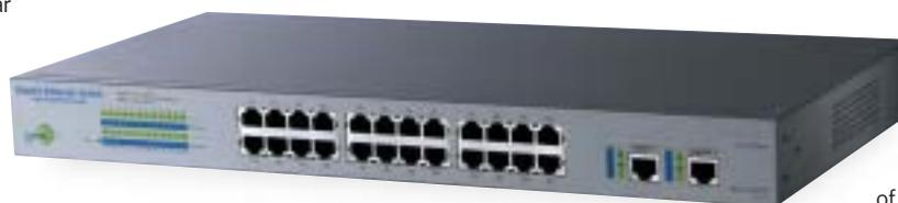
By now, you'll be asking what's the catch – and the answer is in the minimal management tools and features. The Comet Labs GSR224T manages to rise above the status of a dumb, Layer 2 switch thanks to the serial port at the rear.
