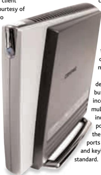
The T20 came equipped with 64Mb of SDRAM memory and Windows NT 4 as the choice of embedded operating system. This offers a wider range of security features and better remote management facilities than Windows CE, but does require a lot more memory.
