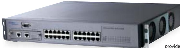
mode and activity. The price for this switch looks steep, but the BPS 2000 is aimed at intensive network applications such as VoIP (Voice over IP) and video streaming, and consequently provides an impressive array of traffic management and prioritisation tools along with good security measures.
