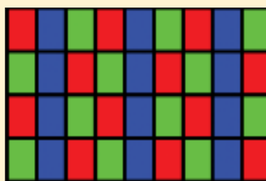
Low-cost PenTile layout.
