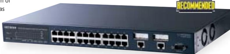
copper, but each port is also paired with a GBIC (gigabit interface converter) slot. These accept industry-standard 1000BaseSX and LX GBIC modules, allowing long-distance fibre-optic connections to be implemented, although the high cost of the cabling limits their value to smaller businesses. The copper and GBIC ports are arranged in pairs, so you can only use one of each and the interfaces must be selected from the management interface.
