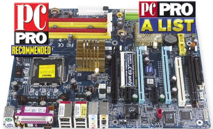
It's just one of the many tricks that the nForce4 SLI chipset has up its sleeve. There's a hardware firewall on the Gigabit Ethernet connection, and the Media Shield RAID controller that will give you performance-enhancing striped arrays or more secure mirrored disks. Gigabyte provides two Ultra ATA connectors should you still have usable parallel interface disks.
