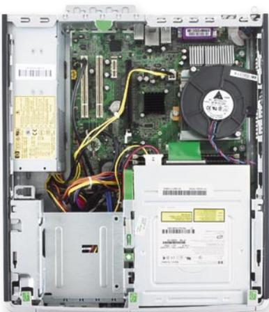
The part of the dx5150's chassis that holds the optical and hard disk drives swings up to reveal a tidy, easy-to-access interior.
