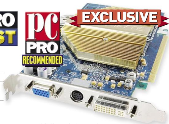
Gigabyte's esoteric naming convention reveals this card to be an X800 XL-based card that holds 256MB of GDDR2 memory for maximum texture storage. The chip itself is based on an 110nm process, allowing ATi to fit more onto a silicon wafer and so cut costs. You can pick up an X800 XL for about £30 less than an X800 Pro. However, thanks to the increased parallelism of the 16 pixel pipelines rather than 12, and the RAM running
