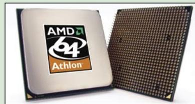
Cool'n'Quiet technology reduces clock speed when demand for computing power is low.
