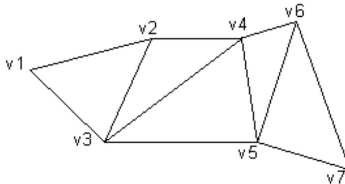
The system uses vertices v1, v2, and v3 to draw the first triangle, v2, v4, and v3 to draw the second triangle, v3, v4, and v5 to draw the third, v4, v6, and v5 to draw the fourth, and so on. Notice that the vertices of the second and fourth triangles are out of order; this is required to make sure that all of the triangles are drawn in a clockwise orientation.
