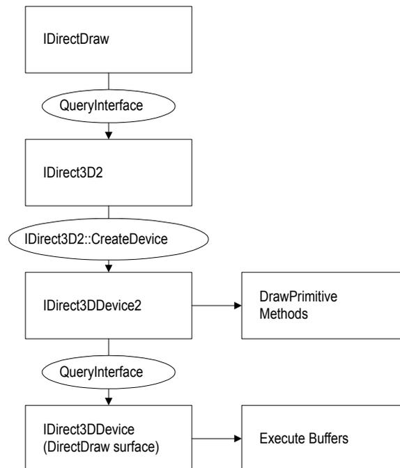
When you create an **IDirect3DDevice2** interface, the Direct3D device object is a separate object from a DirectDraw surface object. The device object uses a DirectDraw surface as a rendering target. This behavior is different from
