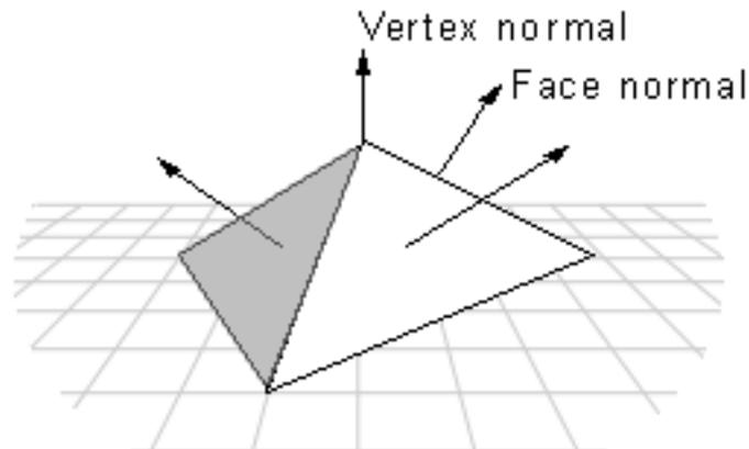
Throughout Direct3D, vertices describe position and orientation. Each vertex in a primitive is described by a vector that gives its position and a normal vector that gives its orientation, texture coordinates, and a color.
