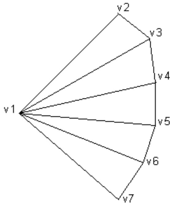
The system uses vertices v1, v2, and v3 to draw the first triangle, v3, v4, and v1 to draw the second triangle, v1, v4, and v5 to draw the third triangle, and so on.
