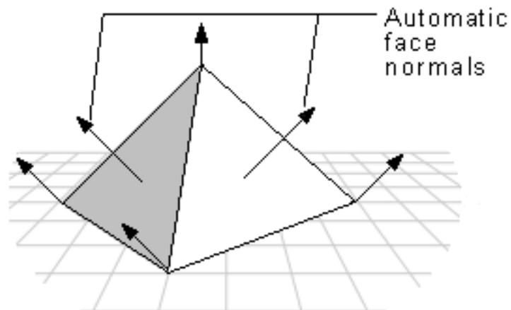
If you want to use the Gouraud shade mode to display curved surfaces and you also want to include some objects with sharp edges, your application would need to duplicate the vertex normals at any intersection of faces where a sharp edge was required, as shown in the following illustration.
