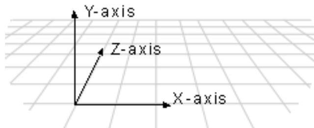
In a left-handed coordinate system, rotations occur clockwise around any axis that is pointed at the viewer.
