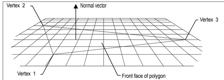
Direct3D applications do not need to specify face normals; the system calculates them automatically when they are needed. The system uses face normals in the flat shade mode. For Gouraud shade modes, and for controlling lighting and texturing effects, the system uses vertex normals.
