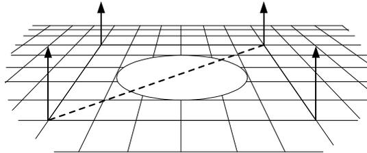
In this case, the Phong shade mode would calculate the value for each pixel and display the spotlight. The Gouraud shade mode, which interpolates between vertices, would miss the spotlight altogether; the face would be rendered as though the spotlight did not exist.
