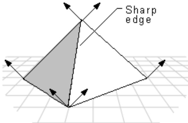
In addition to allowing a single object to have both curved and flat surfaces, the Gouraud shade mode lights flat surfaces more realistically than the flat shade mode. A face in the flat shade mode is a uniform color, but Gouraud shading allows light to fall across a face correctly; this effect is particularly obvious if there is a nearby point source. Gouraud shading is the preferred shade mode for most Direct3D applications.
