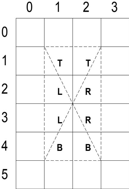
If a rectangle with the same dimensions were moved slightly, so that its upper-left corner were at [1.0, 1.0], its lower-right corner at [3.0, 5.0], and its center point at [2.0, 3.0], the top-left filling convention would be required. Most of the pixels in this new rectangle would straddle the border between two or more triangles.
