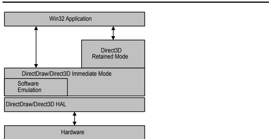
Direct3D is tightly integrated with the DirectDraw component of DirectX®. DirectDraw surfaces are used as rendering targets (front and back surfaces) and as z-buffers. The Direct3D COM interface is actually an interface to a DirectDraw object.
