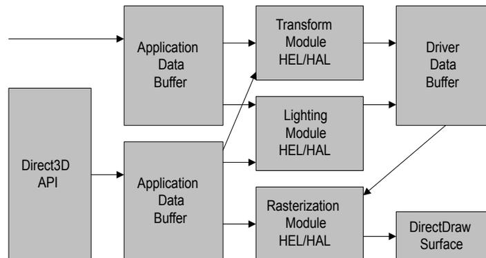
You can disable the lighting module or both the lighting and transformation when you are working with execute buffers. This changes the way the vertex list is interpreted, allowing the user to supply pretransformed or prelit vertices only for the rasterization phase of the rendering pipeline. Note that only one vertex type can be used in each execute buffer. For more information about vertex types, see Vertex Types.
