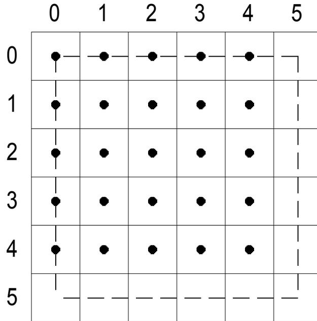
In the top-left filling convention, the word "top" refers to horizontal spans, and the word "left" refers to pixels in spans. An edge cannot be a top edge unless it is horizontal—in the general case, most triangles will have only left and right edges.
