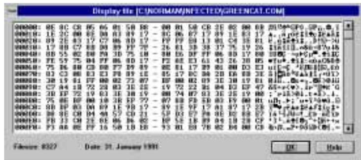
The dialog box shows you the file contents as hexadecimal values (left) and text (right). To maneuver up and down within the file, use the scrollbar along the right edge of the dialog box.
