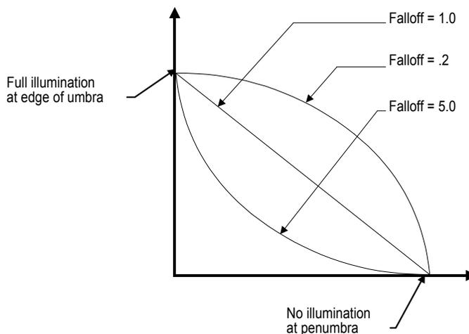
The effect of falloff on the lighting is subtle. Furthermore, a small performance penalty is incurred by shaping the falloff curve. For these reasons, most developers set this value to 1.0.
