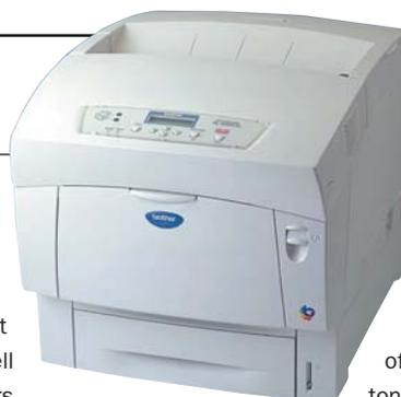
Maintenance of the printer is straightforward, with the integrated printhead cartridge lifting out of the top and the four separate toner cartridges hidden under a removable cover further back. The print cartridge should last for 30,000 pages at five percent cover, while each of the toner cartridges can manage 6,000 (the black one goes on to 8,500). This results in running costs of around 1.3p per black page and 5.8p per colour.
