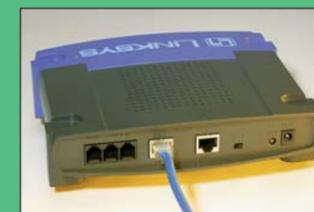
**2** Attach each PC network card (left) to your hub (right) using the special 'crossed' network cable supplied. If you're connecting directly to a PC, you need a crossover cable. This ensures you connect to the right pins and the networked devices can communicate. Once you've connected the access point and hub, you go through the same setup process, but possibly with the additional installation of a gateway to a dialup or broadband modem, so you can use a shared connection
