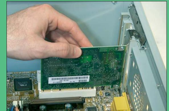
**1** Unscrew and remove the case for each PC that you wish to connect wirelessly. Do this by unscrewing the two or three screws at the back and removing the side panel or the top of the case. Pick a vacant PCI slot for each PC – these are normally the long white sockets
