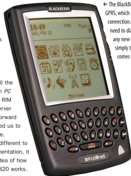
← The BlackBerry 5820 operates over GPRS, which provides an always-on connection. This means there's no need to dial in to check if you have any new messages – new mail simply turns up as and when it comes in
