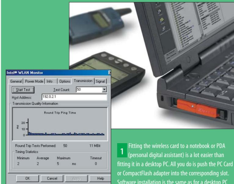
**1** Fitting the wireless card to a notebook or PDA (personal digital assistant) is a lot easier than fitting it in a desktop PC. All you do is push the PC Card or CompactFlash adapter into the corresponding slot. Software installation is the same as for a desktop PC
