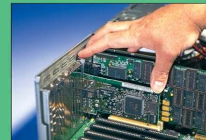
**1** In each PC which is to use the access point, fit a cabled network card instead of the wireless PC Card
