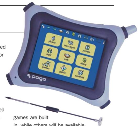
The Pogo is a multipurpose mobile phone that is GPRS- (general packet radio service) ready. It combines email and text messaging, rapid web access, a networked contacts list and diary, MP3 playback and games. Measuring 150x24mm and weighing 243g, the Pogo is large, but this means it offers a spacious touch-sensitive TFT (thin-film transistor) screen. You dial with your finger or the stylus and talk with
