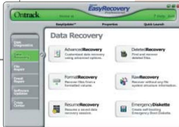
This consists of a set of stripped-down MS-DOS or NT-compatible drivers that enable you to boot your PC from the A drive. You can create such disks in Windows 9x and Me via the Recovery Disk tab in Add/Remove Programs, or by booting from your Windows XP CD and using the Recovery Console by typing `d:/i386/winnt32.exe /cmdcons`, where D is the letter of your CD drive.
