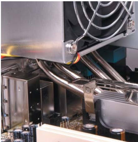
Shuttle's innovative heat pipe solution ensures efficient cooling while cutting down the number of fans necessary keeping the noise low
