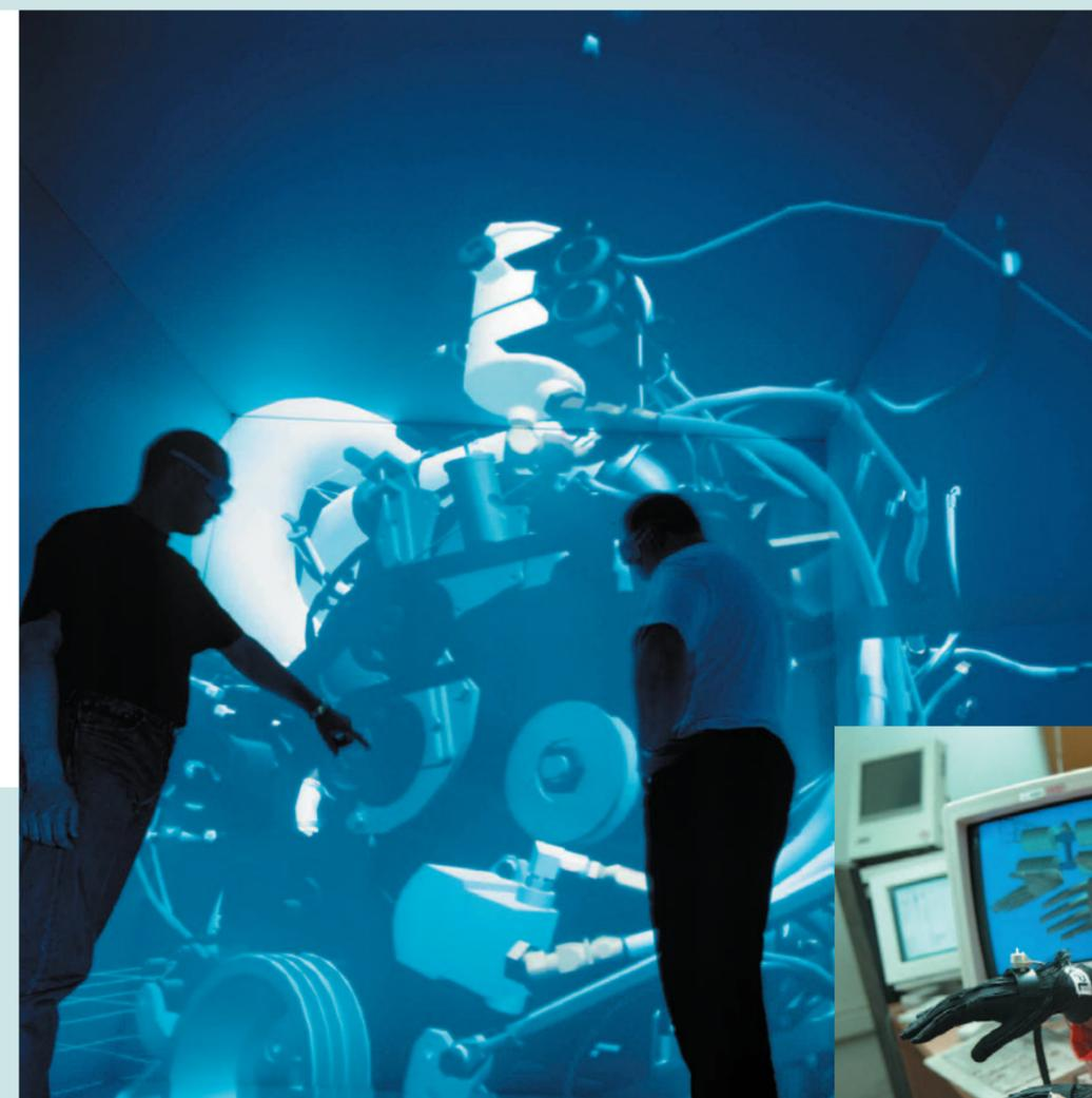
left: the VR Media Lab experimented with Cave technology to produce a VR experience that doesn't require a headmounted display. An entire room is turned into the immersive environment
