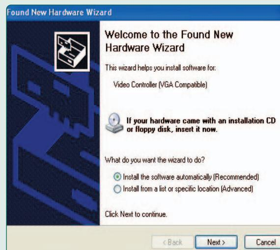
**4** When you reboot your PC the Found New Hardware Wizard should start up automatically. Simply follow the prompts to load the driver. If your graphics card was supplied with an installation disc, click Cancel and use the manufacturer's CD to install the card
