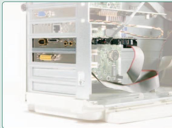
**1** Before installing a new sound card you must eliminate all traces of its predecessor. First, find out whether you have a dedicated card or if sound is integrated on to your motherboard. If you're not sure, use a diagnostic utility such as SiSoft Sandra, shown above.
