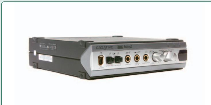
**3** Bundled with the SoundBlaster Audigy ZS Platinum Pro 7.1 is an external box that connects to the sound card via an included cable. The box has a jack for headphones plus digital and analogue input ports for recording music. It's a breeze to install thanks to the detailed setup poster. Boot the PC and install the application software
