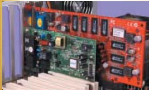
**2** Shut down your computer and unplug the mains lead. Ground yourself by touching a metal object such as a nearby radiator and put on an antistatic wriststrap. Open up your PC's case and remove the screw or retainer holding your existing card in place.
