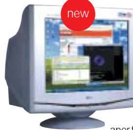
However, the dark and strong image quality generally exhibited by aperture grille technology is considerably toned down here. It's not that the LG's picture is poor, but it lacks the depth of colour of the other aperture grille monitors. It is, however, well suited to close-up work and the 0.24mm dot pitch is possibly a factor in the crystal clear text definition.
