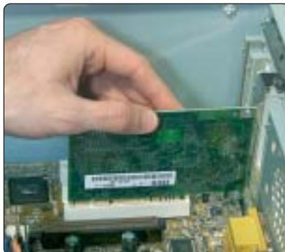
**2** Identify an empty PCI slot and remove the casing's metal strip, if there is one. Put the network card into the chosen slot on an angle and push firmly. When the card is seated in its slot, you can then screw it to the casing in the same place where you removed the metal strip. Replace the computer case cover and plug your network cable into your freshly installed network card
