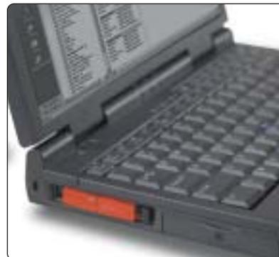
**3** Installing a network card in a laptop is much simpler than a desktop installation. Simply push the credit card-sized card into a vacant PC Card slot. You will most likely have to connect a dongle as well so that the RJ-45 connector can be plugged in. If you opted for a USB ethernet adapter, all you have to do is plug it into a free USB port
