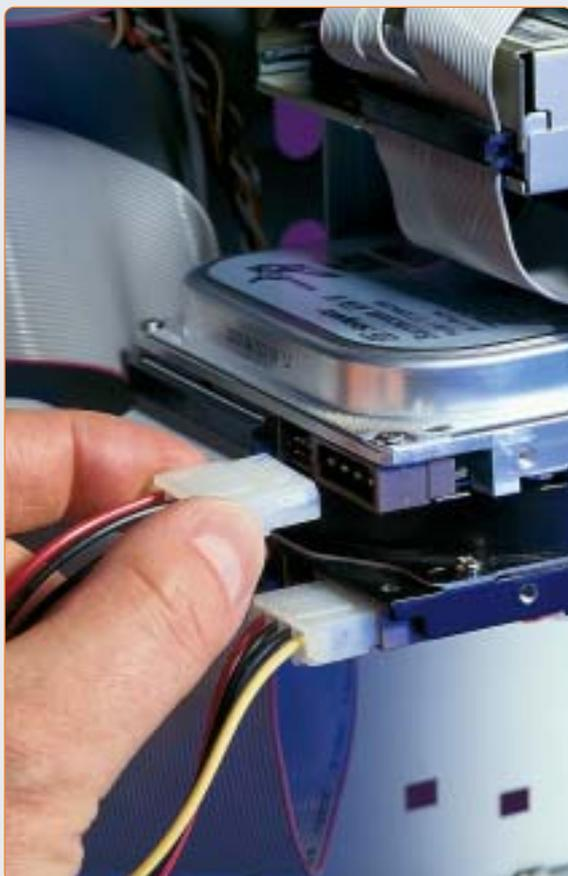
**3 Connect the cables** Most IDE ribbon cables that connect hard drives have two sockets to link a Master and Slave device to the motherboard. If yours doesn't, you can get an upgrade IDE cable. You may wish to purchase a new ribbon cable in any case, particularly if you are replacing your old drive with a faster one.
