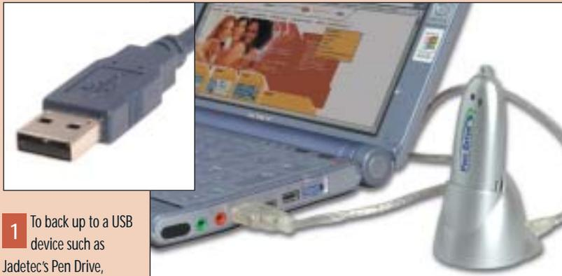
**1** To back up to a USB device such as Jadetec's Pen Drive, install its accompanying software and then connect it via the USB port. Once installed, the Pen Drive appears in Windows Explorer as another drive. Select all the files to be copied and then drag and drop them into the drive's pane
