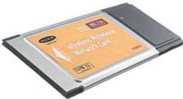
← A wireless network card normally takes the form of an elongated PC Card. It fits directly into a PC Card slot with a small protrusion outside the slot which forms the wireless network aerial
