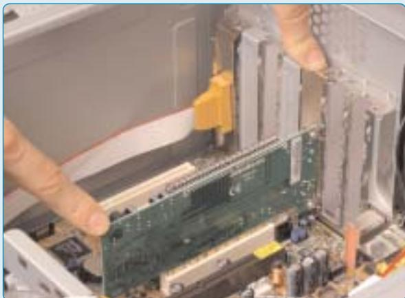
**1** Turn off your PC, disconnect all cables and unscrew the cover. Earth yourself so no static electricity damages your PC's components. Locate a spare PCI slot next to the graphics and modem cards on the motherboard and remove the blanking plate so the card's connectors will be accessible once the PC case is replaced. Ease the TV tuner card into position and push down firmly so it is properly connected. Use the retaining screw from the blanking plate to secure the card
