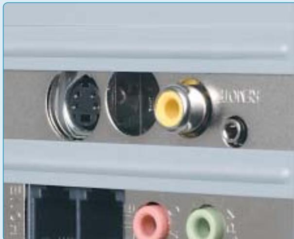
**2** Replace the PC cover, reattach all cables and peripherals. If the tuner card came with a remote control attach its infrared cable to a free USB port, ensuring the other end sits somewhere in line of sight so the controller can communicate with your PC. Attach the TV aerial and any signal boosting devices. Restart the machine and install the TV tuner and TV interface software
