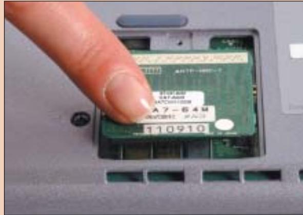
**2** With the notebook switched off, the case open and wearing an antistatic wriststrap, hold the memory module by its edges, taking care not to touch the gold connectors on the chip itself. Fit the row of pins on the chip to the row on the motherboard, then press it firmly into place
