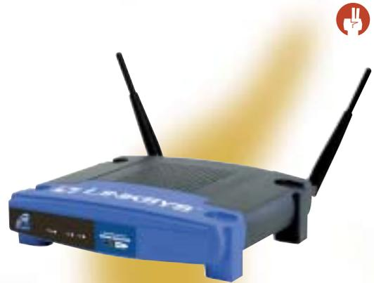
↑ Wireless broadband routers connect to your always-on internet connection and then allow all local computers around with wireless cards to access the link. The router will firewall the link, allowing you to share drives and folders safely around the network
