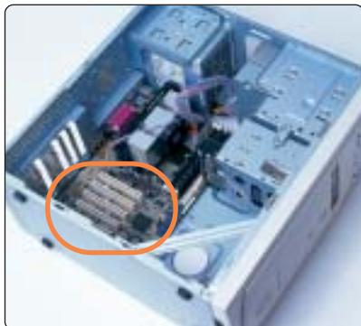
**1** Unplug the power, remove the casing (use a screwdriver if you need to) and identify the PCI slots: they are generally white and the only type into which your card will fit. Older computers will have a couple of ISA slots as well as a few PCI slots and some of these will already be occupied. Before putting the network card into the PCI slot, ground yourself by touching any of the metal surfaces on your computer casing. This will discharge any static built up in your body or clothing
