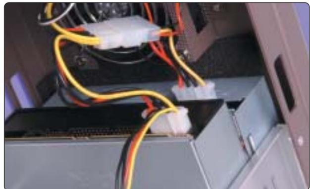
**3** Grab the drive's cable and plug it into any of the white connectors from the multicoloured bundles of wires protruding from the power supply unit. You'll probably also need to plug one of these connections to the fan connector built in to your PC's casing before reassembling everything, powering it up and installing any accompanying software. Our TDK device came with Sonic's MyDVD, an easy-to-use package bundled with many DVD writers
