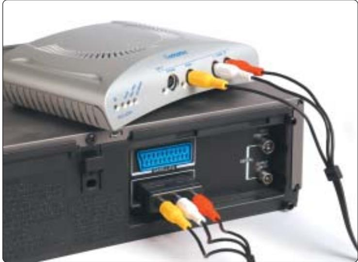
**2** If you don't have the three-way video-out connections described, you can emulate them using a Scart adapter (available at most electrical stores). With connections made, plug the external capture box into a free USB slot on your PC. Load up the bundled Sonic MyDVD software (or other video-editing software if it's compatible with Mpeg-2 capture) and start the videotape to begin the transfer process
