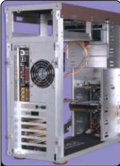
There's a series of metal cages behind the case's front panel where you attach various drives. The narrower cages are for hard disks and floppy drives, while the wider ones are for optical drives such as DVD-ROM and CD writers
