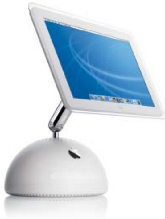
➤ Processor, memory, drives and power supply are all squeezed into a compact round base which measures just 10.6in in diameter
