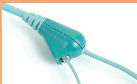
**2** For the point where the USB modem is to be attached, connect a filter to the wall socket and insert the turquoise data cable into the DSL socket. Unless you have a splitter at this point, the Phone socket will be unused
