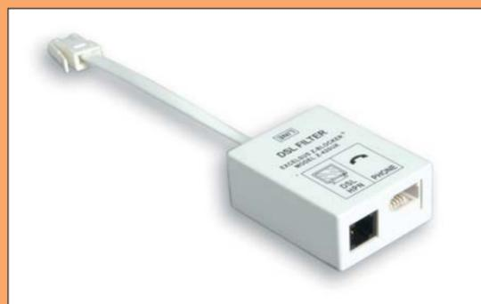
**1** Disconnect the phone jack from the wall or extension socket and insert the tail of the ADSL filter instead. Then put the original cable into the socket marked Phone on the filter. Splitter sockets can also be used. Again, insert the jack into the Phone socket on the filter
