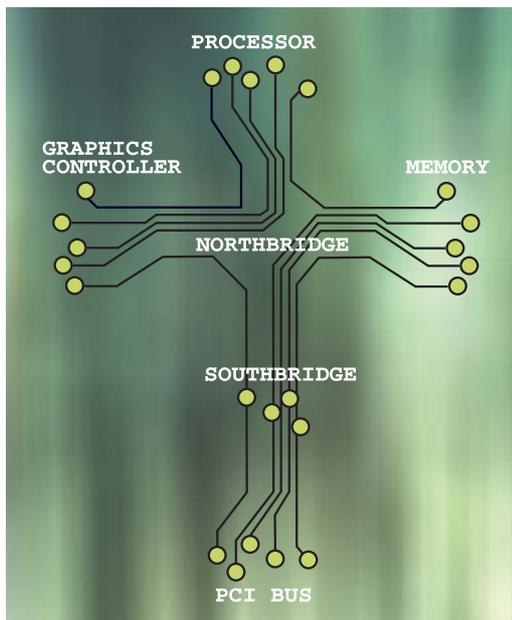
slots on the motherboard for expansion cards, providing a communications link to the rest of the system). All these components need to talk to one another. The north bridge is the central component, connecting together the processor, memory, graphics controller and the south bridge, with the PCI bus communicating through the south bridge. Other motherboard components, like USB and network ports, also connect through the south bridge.
