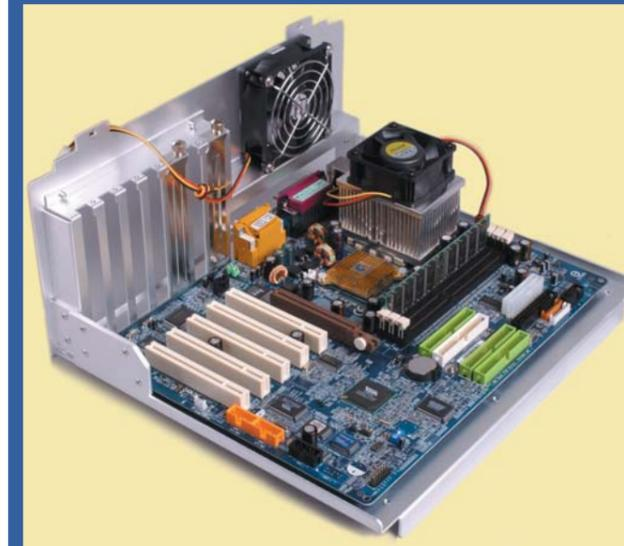
The motherboard would shortcircuit if it were placed directly into a PC case, so it's held just above the surface by a number of small plastic or metal spacers that are supplied with the case. Ensure these are clipped or screwed into the holes in the case so they line up with the holes in the motherboard's surface – ours need about eight to keep them firmly in position. Finally, lower the motherboard gently on to the spacers and screw it in place.
