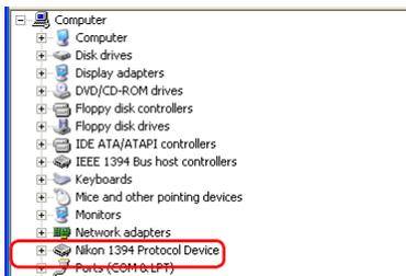
2 Double-click the listing for your camera to open the device properties window. If the camera is listed under “Other devices,” [re-install the device drivers](#). If “Nikon 1394 Protocol Device” is not listed in the Device Manager and the camera does not appear under “Other devices,” disconnect the camera and restart the computer. Reconnect the camera after the computer has restarted.
