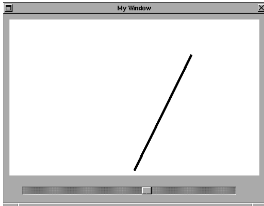
Figure 8-7: Controlling some aspect of drawing with a slider
