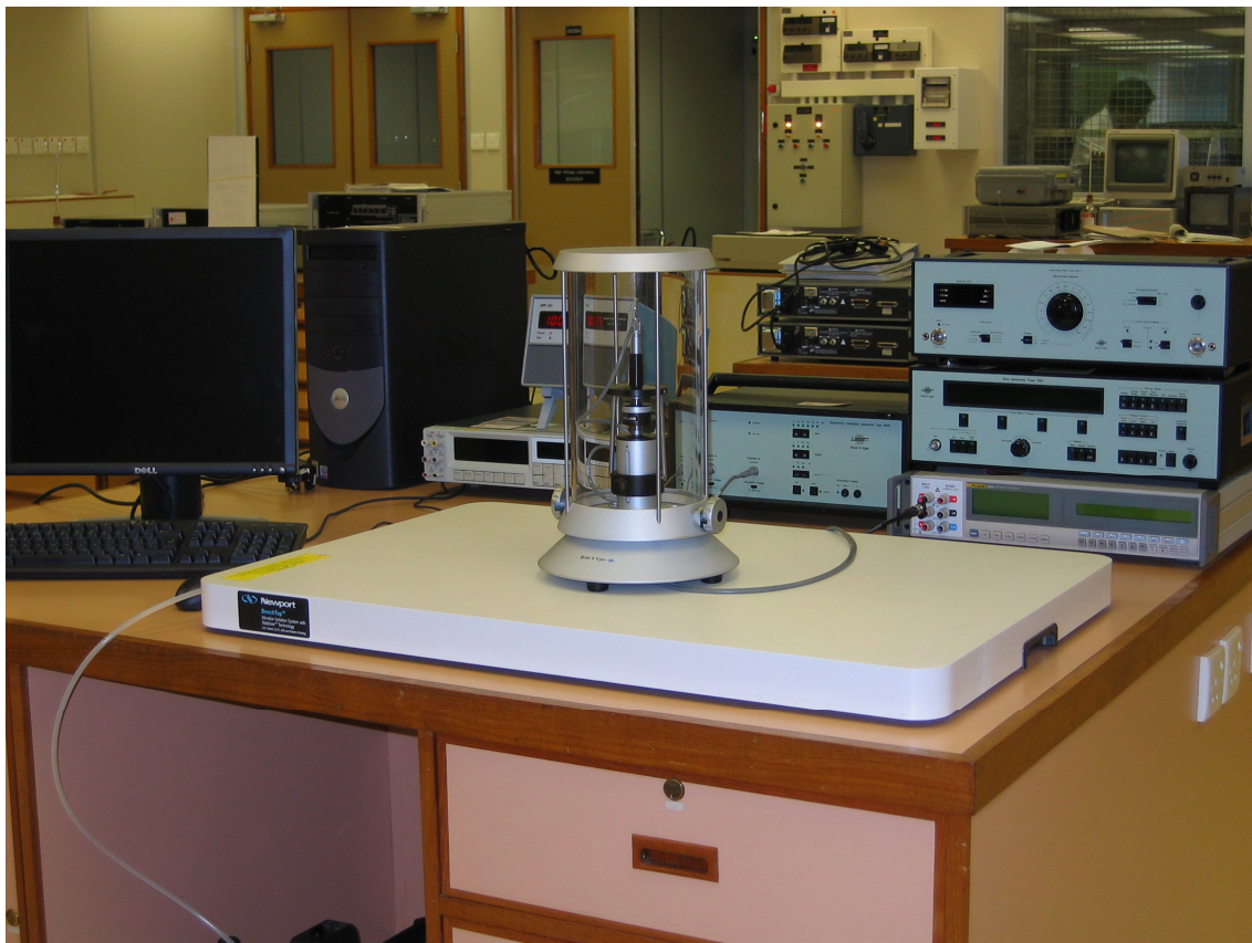
Figure 2 - Reciprocity calibration system for laboratory standard microphones.
