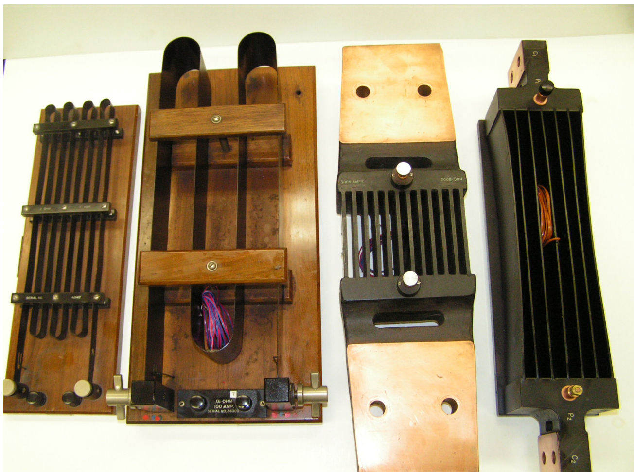
Figure 2. Shown from left to right are a 0.1\ \Omega / 15\ \text{A} ribbon shunt, a 0.01\ \Omega / 100\ \text{A} ribbon shunt, a 10\ \mu\Omega / 3000\ \text{A} parallel element shunt, and a 100\ \mu\Omega / 1000\ \text{A} parallel element shunt.
