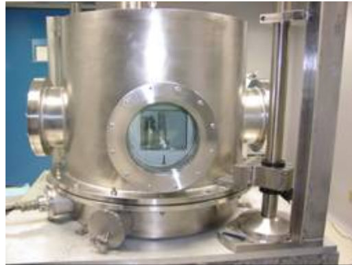
Figure 2. The air-tight chamber, the HK 1 000 MC mass comparator is installed inside
