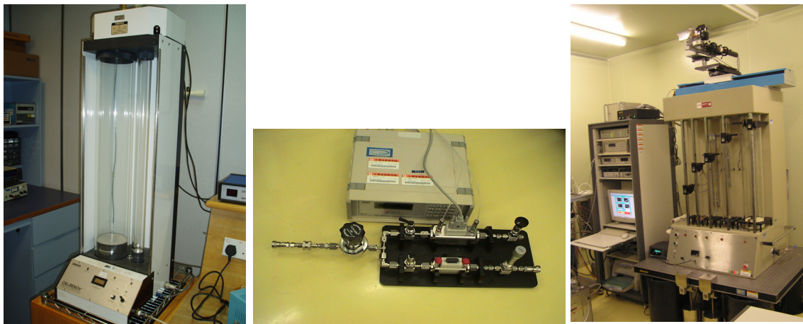
Figure 1. Flow systems for inter-comparison and LFE transfer standards.
