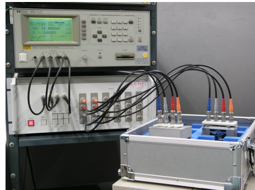
Fig. 4 Connected circuit for LCR meter and coaxial scanner
