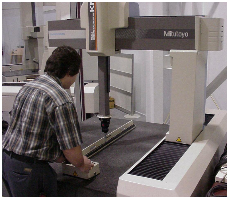
Figure 2. Testing length measuring accuracy on a CMM.
