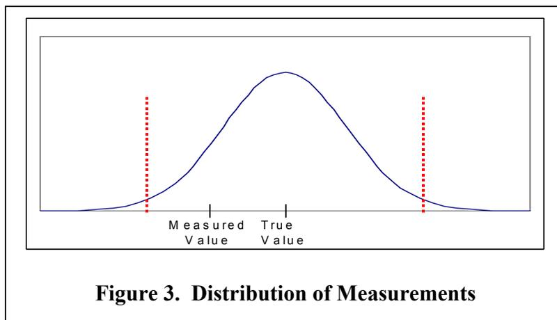
The distance from the true value to the dashed lines characterizes how big a measurement error could be and is called the uncertainty. Note that the uncertainty is not a specific measurement error, but rather helps to establish a range of values for the error. So we could say that
