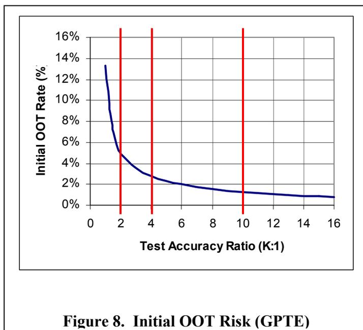
As can be seen in Figure 7, having a low TAR between the calibration standard and the test equipment will cause a lot of unnecessary calibration (adjustment). However, the larger risk is in sending the Navy out-of-tolerance test equipment. With a 2:1 TAR, it can be seen in Figure 8 that nearly 5% of the test equipment will be initially out-of-tolerance. The required 4:1 TAR improves this to less than 3%, while a 10:1 TAR drops the risk to nearly 1%.
