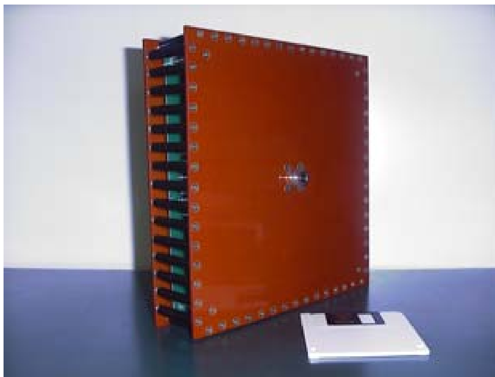
Figure 1. Developed AC shunt.
