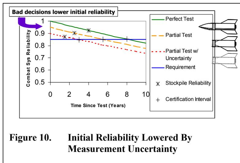
**Figure 10. Initial Reliability Lowered By Measurement Uncertainty**
