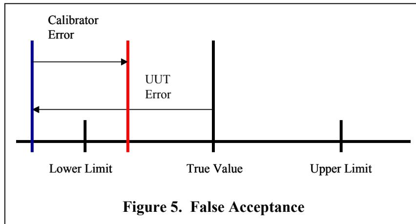
In a false accept, the UUT really is Out of Tolerance, but the Calibrator Error brings it back In Tolerance. The probability of a false accept (PFA) is given by:
