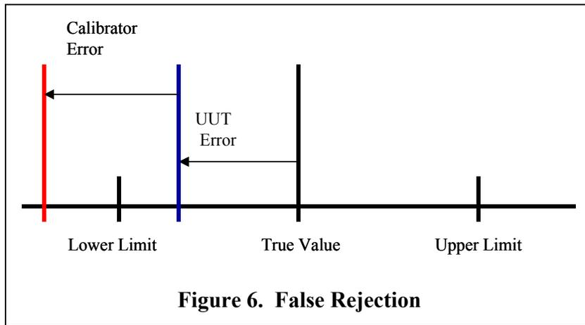
In a false reject, the UUT is really In Tolerance, but the Calibrator Error moves the comparison Out of Tolerance. The probability of a false reject (PFR) is given by:
