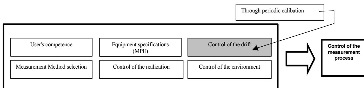
The intent of periodic calibration is to limit the drift of the equipment (drift must be understood either continuous or erratic). What is important for decision making about periodicity is the ratio : Drift / product tolerance and can be expressed as the product of 3 ratios :
