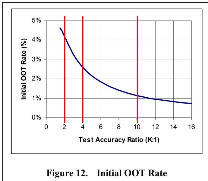
With a 4:1 TAR, approximately 14% of the test failures will be due to the test equipment rather than the tested system. This means that 14% of the repair and maintenance work done as a result of the testing will be unnecessary. By increasing the TAR to 10:1, we can decrease the unnecessary rework to as little as 5%. In cases where the TAR is 2:1 or lower, the percentage of unnecessary rework skyrockets to 31% and more.
