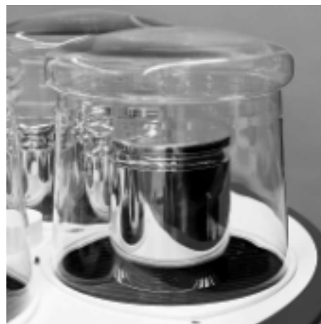
Figure 6: Individual glass covers protect the loads from air drafts.
