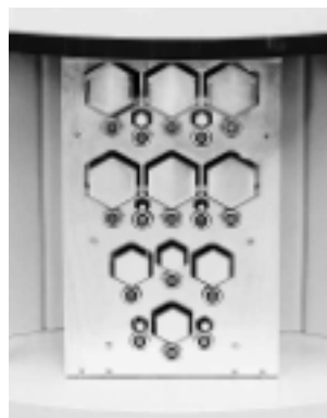
Figure 2: Front view of the comparator's substitution weight set.
