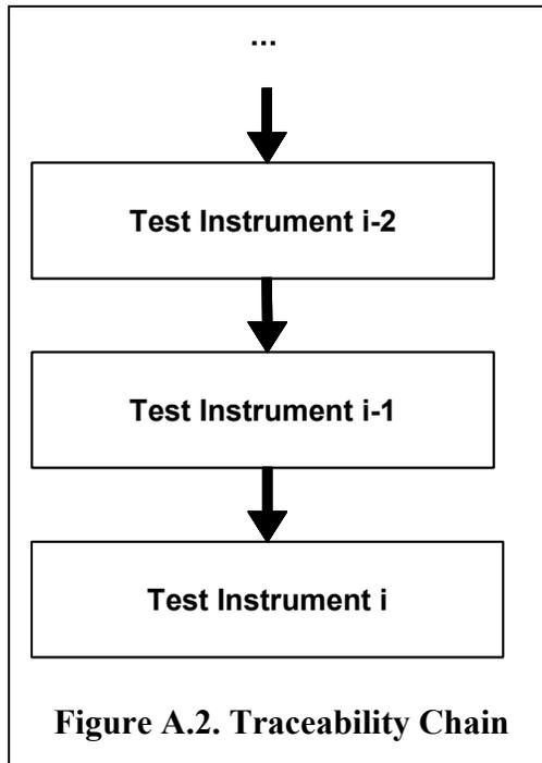
In a calibration scenario, there is a calibrator and a unit under test, or UUT. The UUT will be given the subscript  $i$ , where  $i$  could take values from 1 to  $N$ . The calibrator, being the next test instrument up in the chain will generally be given the subscript  $i-1$ . The measurement model for the UUT will be given as:
